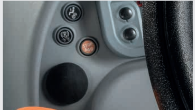
↑ Stop&Go function lets the driver stop and hold the tractor without using the clutch pedal.
