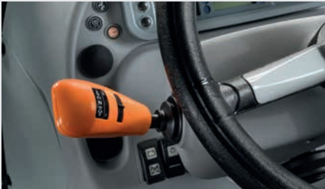
↑ PowerShuttle with SenseClutch (5 adjustable levels).
