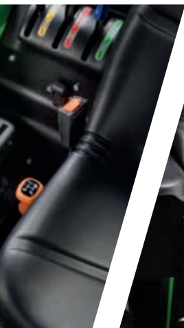
> 3 rear spool valves with quick couplers.
