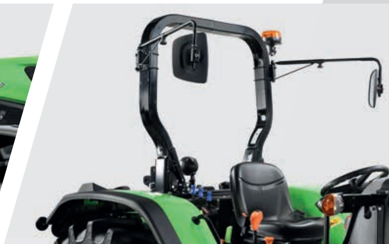
> Rear mirrors installed on ROPS.
