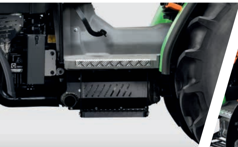
> Fully integrated EAT system. SCR and DPF installation does not impact on mudguards height and bonnet dimensions.
