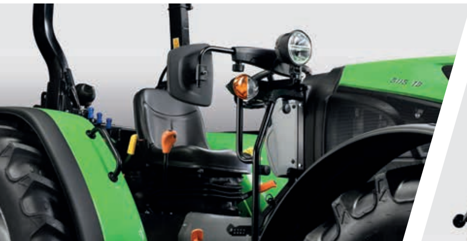
> Rear mirrors installed in the front of the platform.
