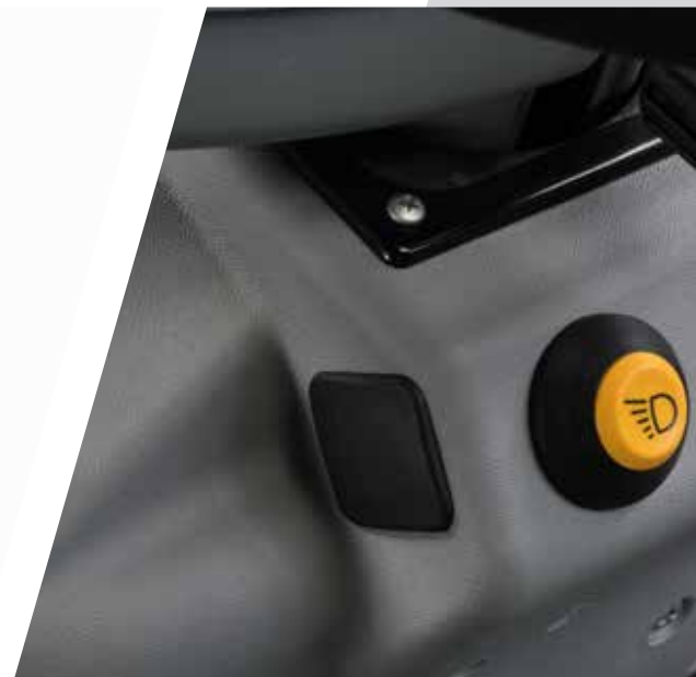
> SDD function, halves the numbers of steering wheel turns for complete steering.
