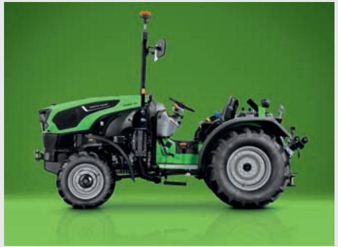
↑ All models are available as platform version with 2-post foldable safety frame.
