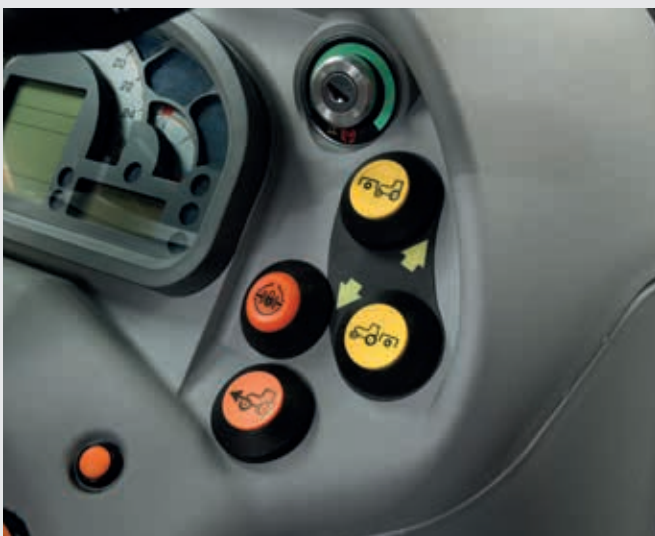
↑ Easy engagement of front and rear PTO through ergonomic buttons.
