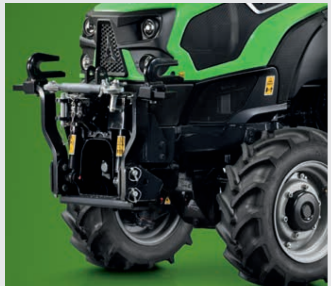
↑ Fully integrated front lift and front PTO.
