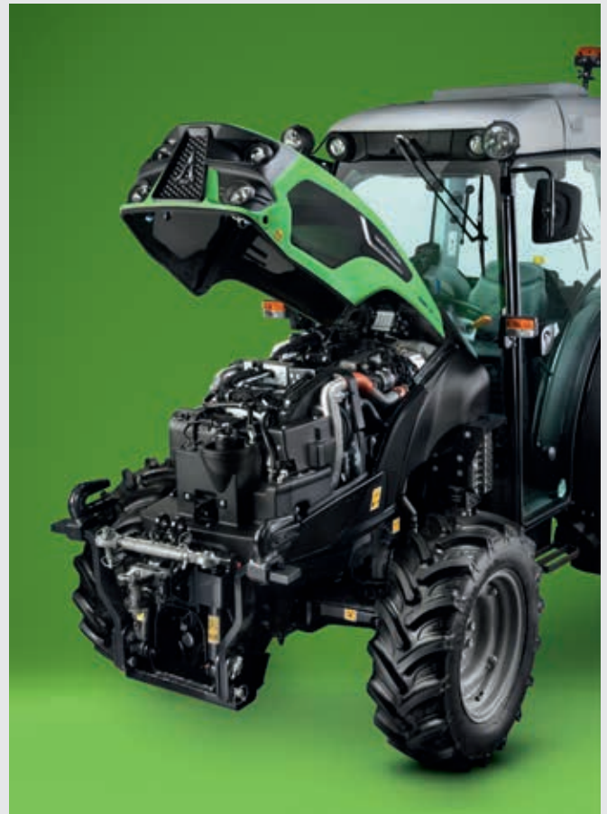
Stage V compliant through a simple EAT system. AdBlue not required.
