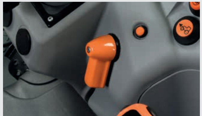
Electronic engine governor with one engine memory speed.
