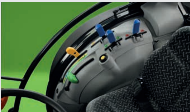
↑ Simple and effective mechanical rear lift control.
