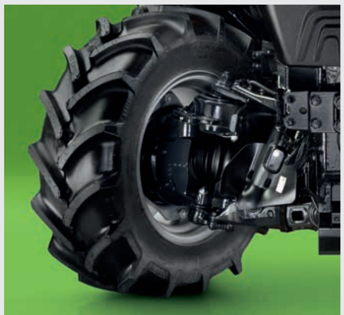
↑ Independent front axle suspension available on all models.
