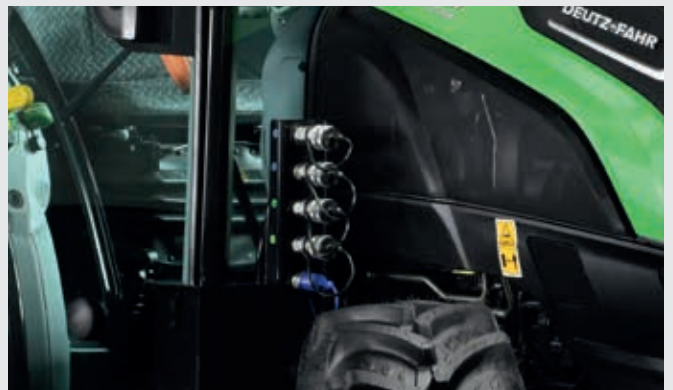
⬆ Up to 4 mid-mounted hydraulic ways and 1 free return.
