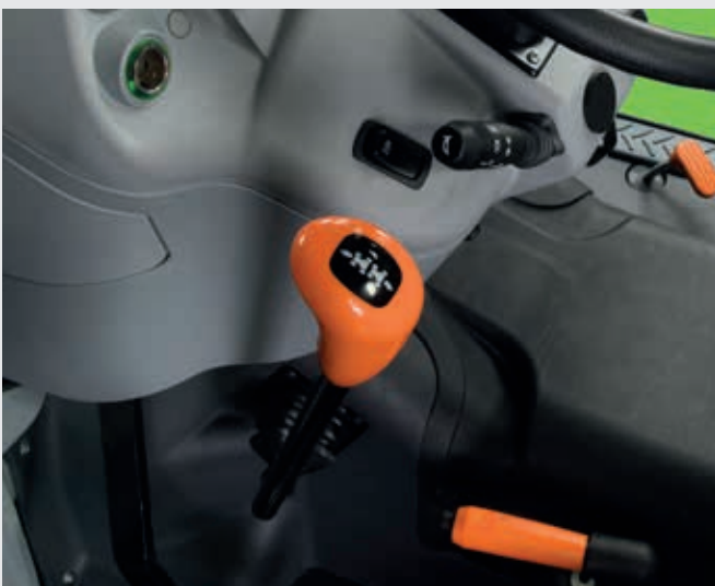
↑ Mechanical shuttle lever on steering column.
