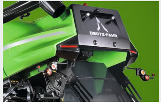
↑ Big straw-hood discharge chute to maximize the product flow of the long straw.
