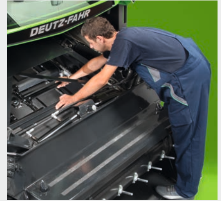
↑ Easy access to adjust and check the chains on the feeder channel.
