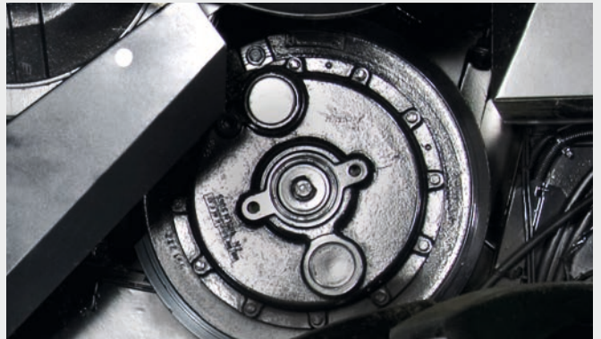
↑ Optional threshing drum speed reducer to set the threshing drum rpm from 1250 to 625 as maximum speed and from 420 to 210 rpm as minimum speed. This kit is suggested while harvesting maize.
