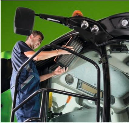
↑ Tool free dismantling of the air filters of the cabin.
