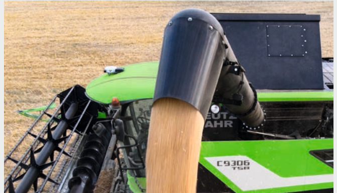
Integrated light and camera on the unloading pipe to check the unloading operations.
