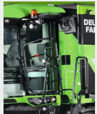
Dual inspection window in the cabin, easy sample pick up tray just outside the cabin.
