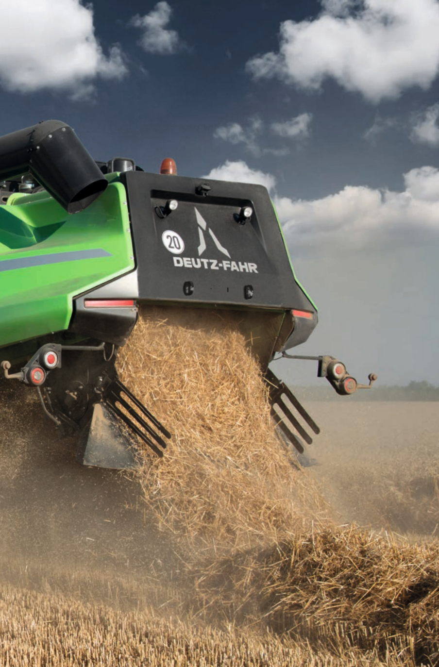
↑ Big straw-hood discharge chute to maximize the product flow of the long straw.
