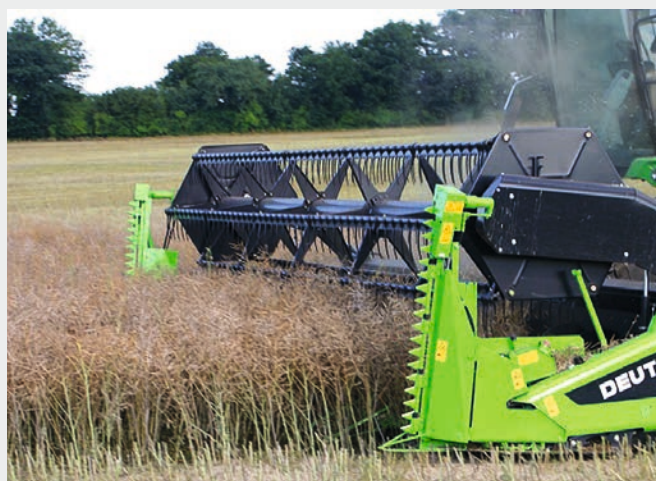
↑ For rape harvesting there is a specifically designed kit which can be applied to the standard DEUTZ-FAHR headers up to 7.2 m.
