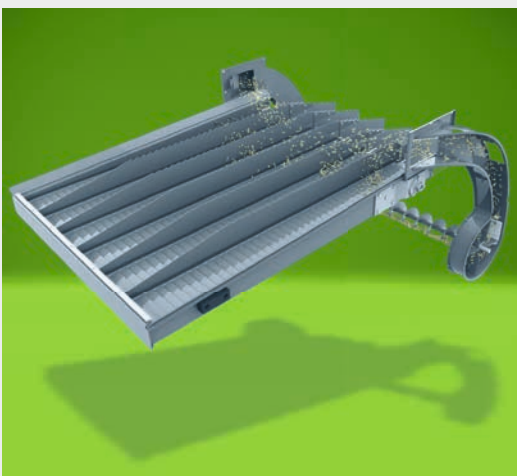
↑ DGR System: returns elevators on both sides of the machine with special friction plates to thresh the crop while returning it onto the preparation pan.
