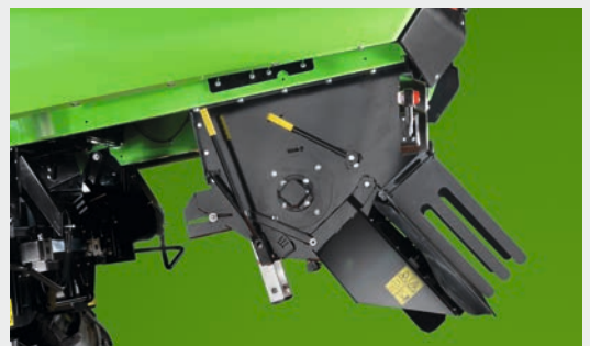
↑ Straw-chopper unit with spreader adjustable in 3 positions. The spreader unit is converted to a chute for the long straw while not in use.
