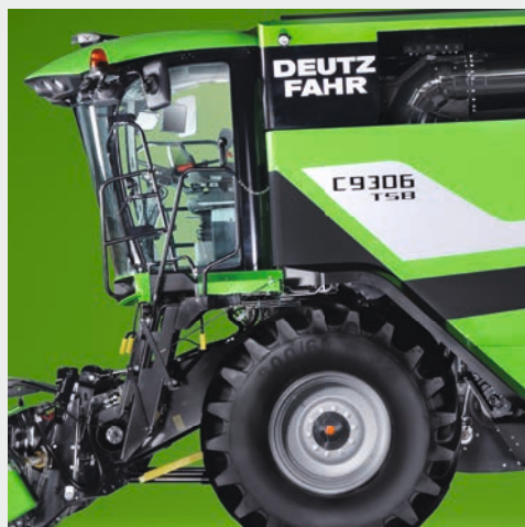
↑ Easy access to the cabin thanks to the new ladder with automatic folding and unfolding system.
