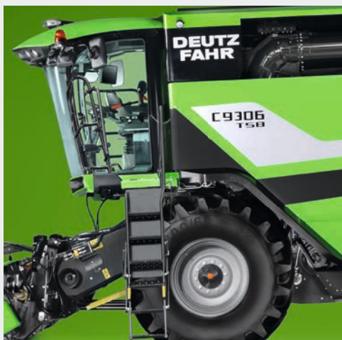
↑ Easy access to the cabin thanks to the new ladder with automatic folding and unfolding system.
