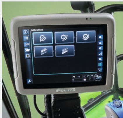
↑ Perform and control the calibration of all main systems directly from the iMonitor.
