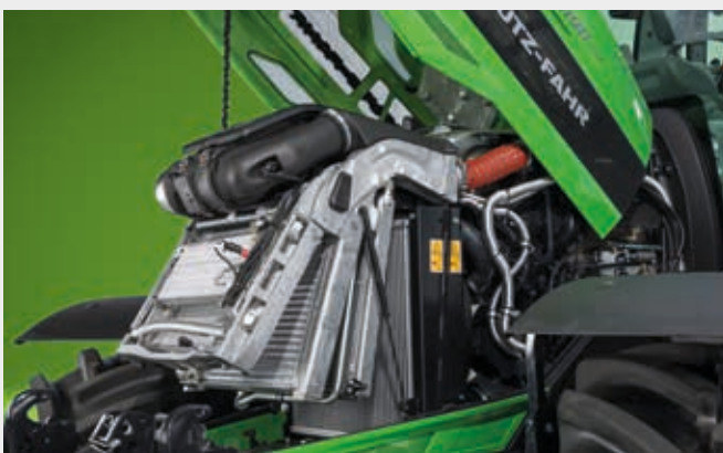
↑ Aluminium cooling system of 6190 TTV with one-hand access lever and Powercore air filter.
