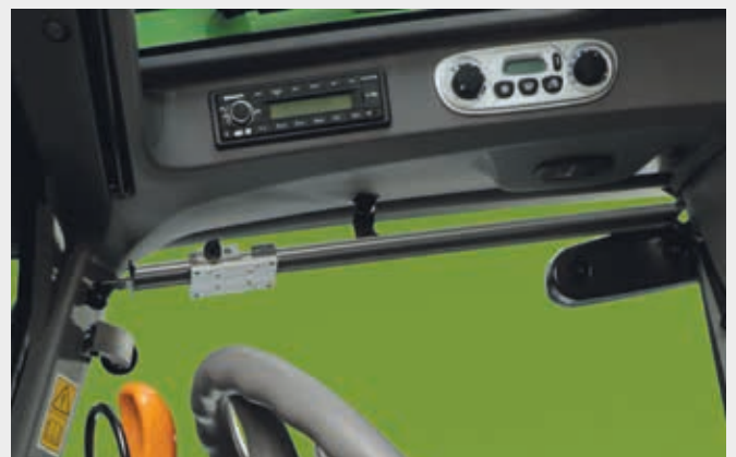
↑ Radio, AC and lights control interfaces as well as sliding monitor mount.
