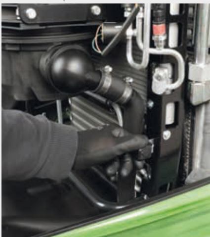
↑ Cooling package with easy opening mechanism.
