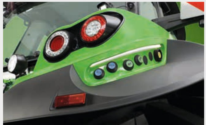
Illuminated push buttons for external control of the rear lift, the PTO and a spool valve.
