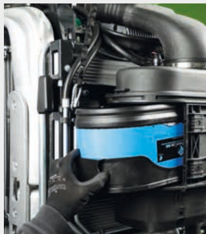
↑ Airfilter with pre-cleaning unit.
