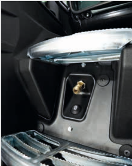
↑ Air supply port and entrance light switch protected under the steps.
