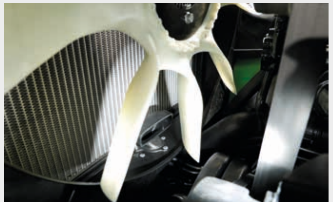
↑ Electronic viscstatic fan (eVisco) with suction hose for the air filter pre-cleaning system (removes 95% of coarse particles before they can reach filters).
