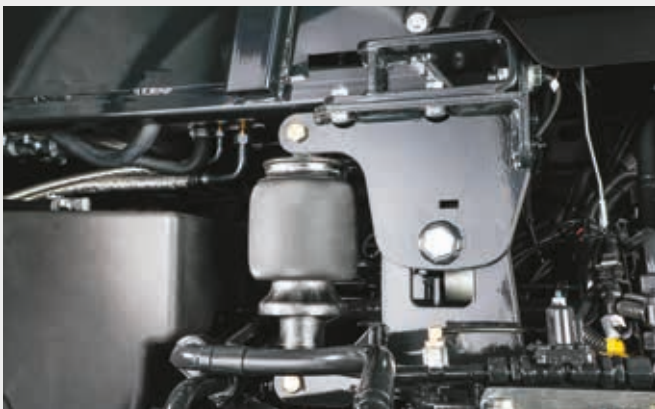
↑ Air spring elements of the comfortable air suspension of the cab.
