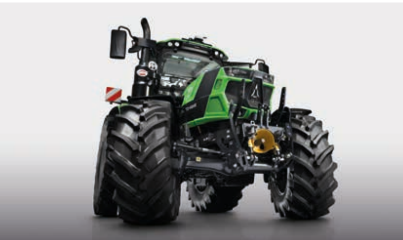
> Front suspended axle with 100% front differential lock.
