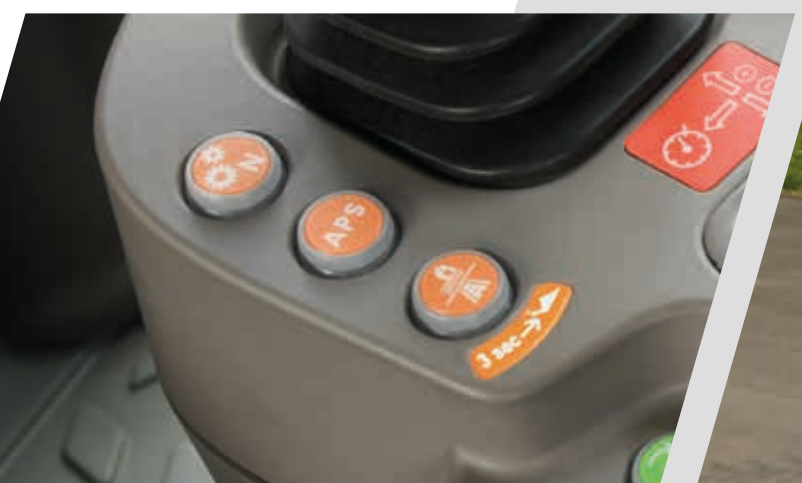
> Selection of Transport, Field and Creeper driving modes.
