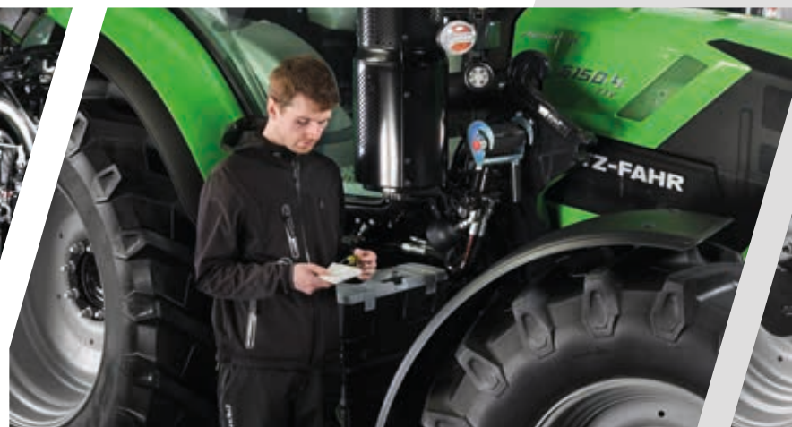
> The engine oil dipstick is accessible without opening the bonnet.
