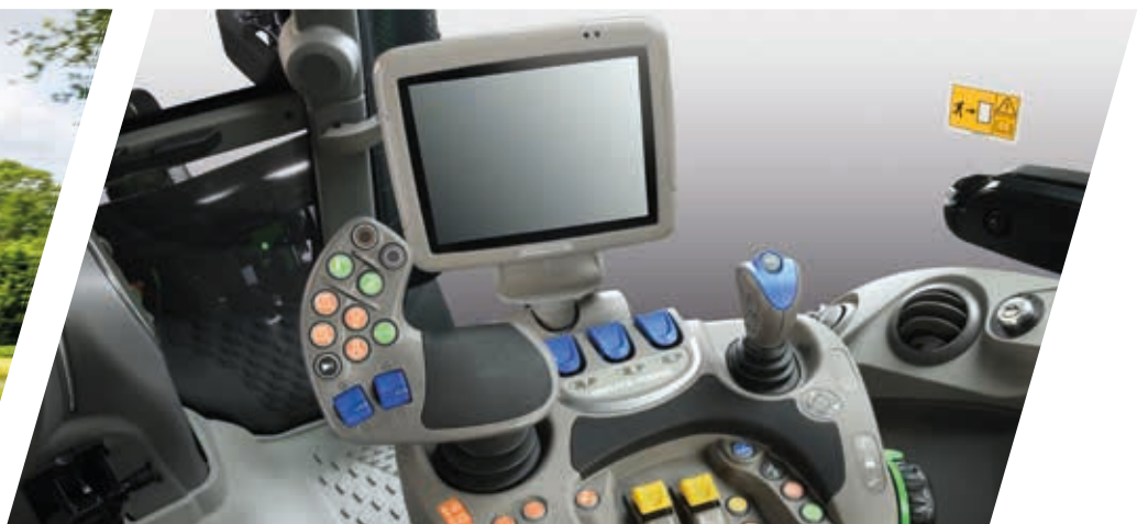
> Ergonomic MaxCom joystick with lift buttons, engine/transmission controls, headland management button, two proportional hydraulic valve control units and two freely assignable Jolly buttons.
