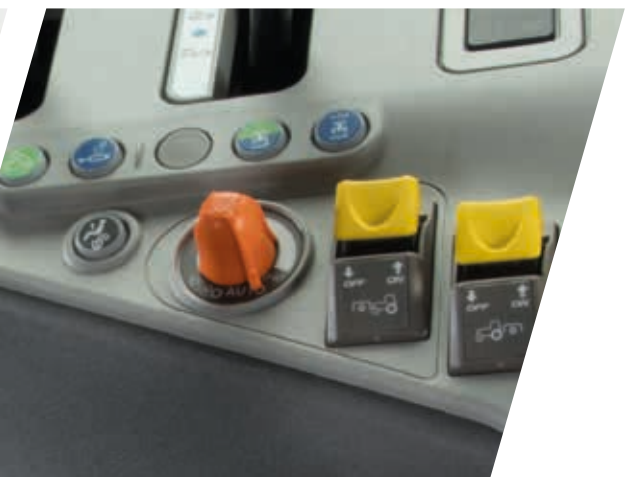
> Easy and intuitive – with the ECO/Power adjustment knob the operator can change the APS (Automatic Powershift) shifting behaviour.
