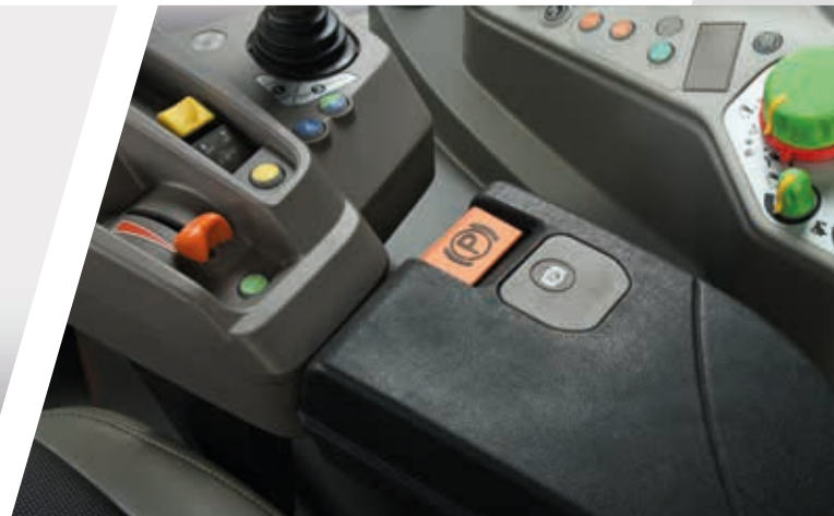
> Electronic Park Brake (EPB) on RVshift and TTV models.
