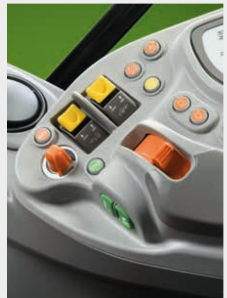
↑ Front and rear PTO electrohydraulically engaged and AUTO PTO function.
