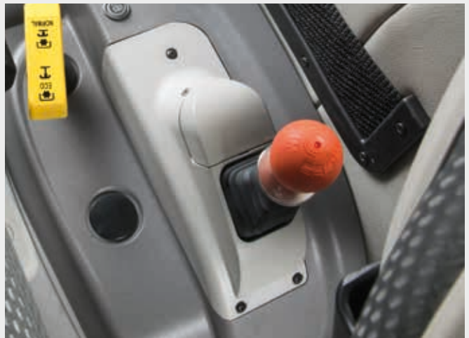
↑ HPB (Hydraulic Parking Brake).
