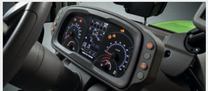
↑ Analogue-digital dashboard with main tractor functions at a glance.
