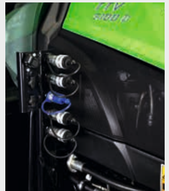
↑ Mid-mounted hydraulics ways for front implements.
