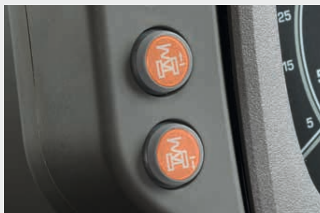
↑ Two new dedicated buttons allowing manual adjustments of the position of the front suspension.
