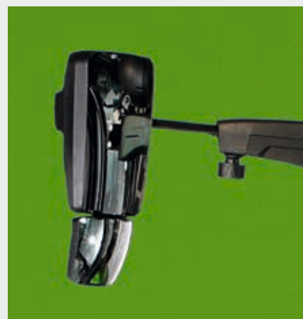
↑ Mirrors with electric adjustment and defrosting.
