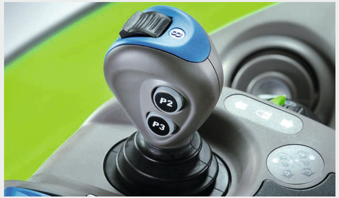
↑ The cross-control lever with rocker switch controls three hydraulic control valves.
