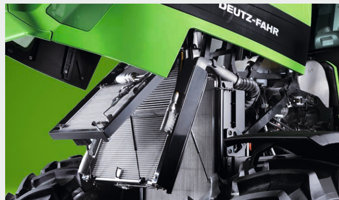
↑ The engine radiator can be opened and cleaned easily.
