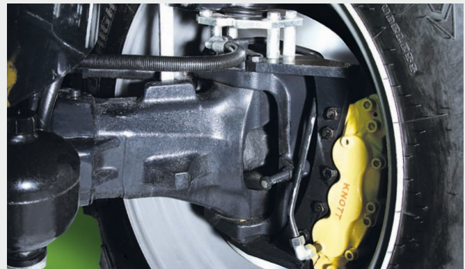
↑ Dry disc brakes on the front axles for extra safe brake action (optional).
